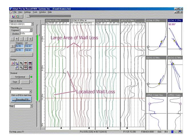
or ease of use, the probe comes with its own probe definition file which allows the user to instantly configure the Adept Pro analysis software for the collapsible probe. Because the probe connects directly to the Ferroscope 308 system, no separate hardware setup is required.
